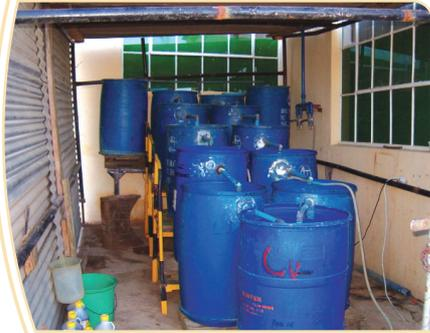
A jaw crusher is used to crush the ore, which is then ground fine by a hammer mill. The first picture is that of the 'raw ore', before it is ground into a fine 'powder'. The other two pictures are the leaching equipment/circuit, where the copper is leached from the ore using a sulphuric acid solution. The concentrated copper solution is used to electroplate copper onto wax moulds resulting in the creation of copper artefacts, which are sold to tourists and other companies in the region.
